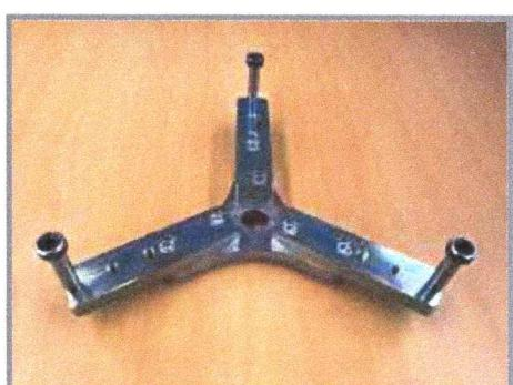
6. Assemble the wrench of the bladder dismantling tool.
