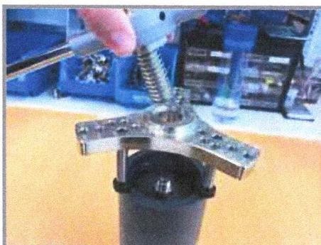
8. Introduce the wrench axis of the tool through the central hole of the star frame and screw the threaded extreme of the axis in the charging valve or adaptor ¼" BSP previously threaded on the top lid.
