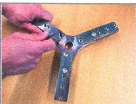
5.1 Screw the 3 legs included in the kit into the corresponding female threads of the star frame. Place the legs according to the model UXXX which is going to be dismantled. The model number UXXX is engraved in the female threads of the star frame or extensors.
