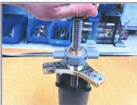
9. Rotate the two wrench arms clockwise to extract the top lid from the damper housing.
