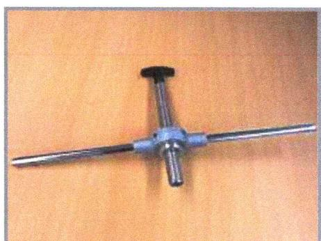
7. Place the star frame (with the screwed in legs) above the bladder pulsation damper. Legs ought to be leaning in the pulsation damper walls.
