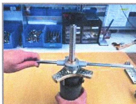
10. Once the top lid has been extracted, the bladder can be easily disassembled from it. The pulsation damper is now completely disassembled.
