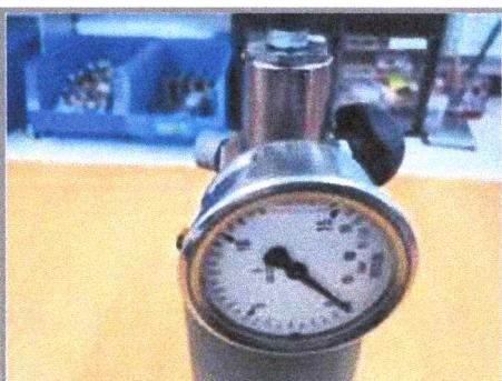
If the pulsation damper is charged at a low pressure (below 10 bar), it will be enough to release the gas from its interior by pushing the core of the charging valve with the help of an awl.
