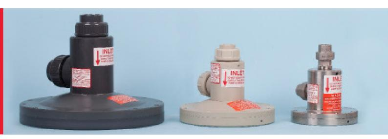
The Series 2100 suction demand valve (SDV) is designed specifically for the dosing industry to hydraulically isolate a metering pump from its bulk supply tank, preventing variations in suction pressure and pump accuracy. The valve will prevent uncontrolled discharge from the storage tank in the event of a pipeline rupture downstream of the valve.
