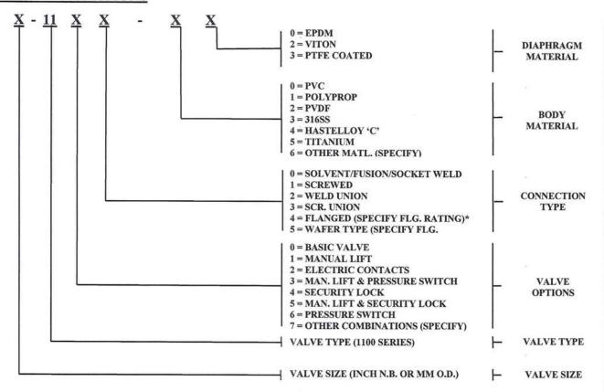
**DUPLEX VALVES -** Add the letter 'D' after the valve designation. **SPECIAL CONFIGURATION VALVES -** Add suffix'X' after total designation and specify features.
